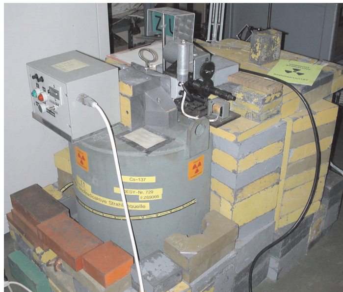
Figure 9.4: The ^{137}\text{Cs} gamma source.
