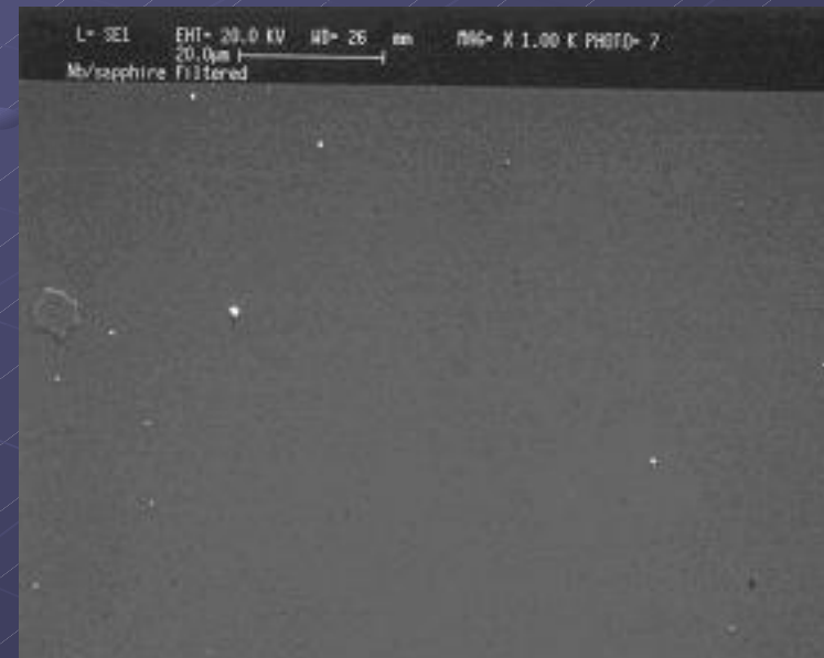
Surface of the Nb coating obtained with the use of the filtered UHV arc
