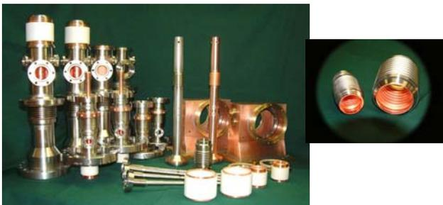
Fig. 6: Photographs of the different copper-plated parts of TTF3 coupler
