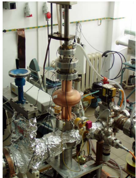
Fig. 3 UHV system with a linear-arc.
