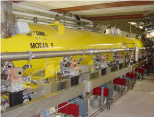
Figure 2: Accelerating module in the VUV-FEL tunnel.
