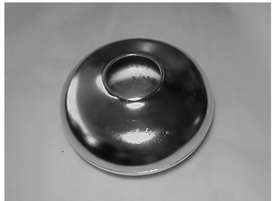
Fig.2. TESLA type copper cavity, which was coated with a pure Nb layer at IPJ in Swierk.
