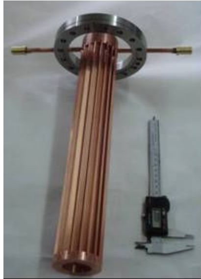
Fig.4.1.3. View of the cylindrical Venetian-type micro-droplet filter.
