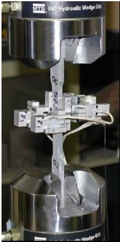
Fig. 2.2.1: Experimental tensile tests on an Al specimen alloy.
