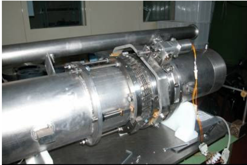
Figure 8.1.2: Complete assembly provided with leverage mechanism and stepping motor.
