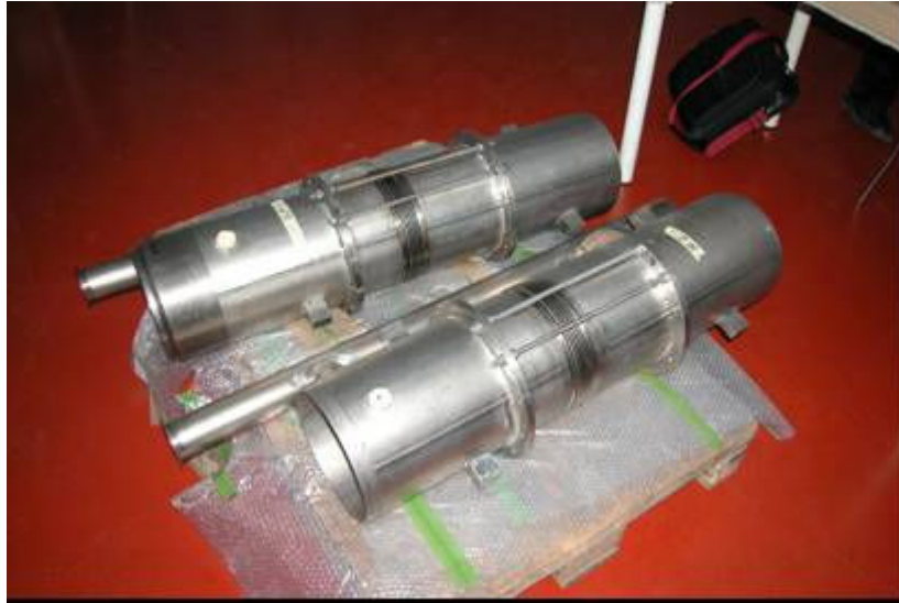
Figure 8.1.1: TTF cavities modified Helium tanks
