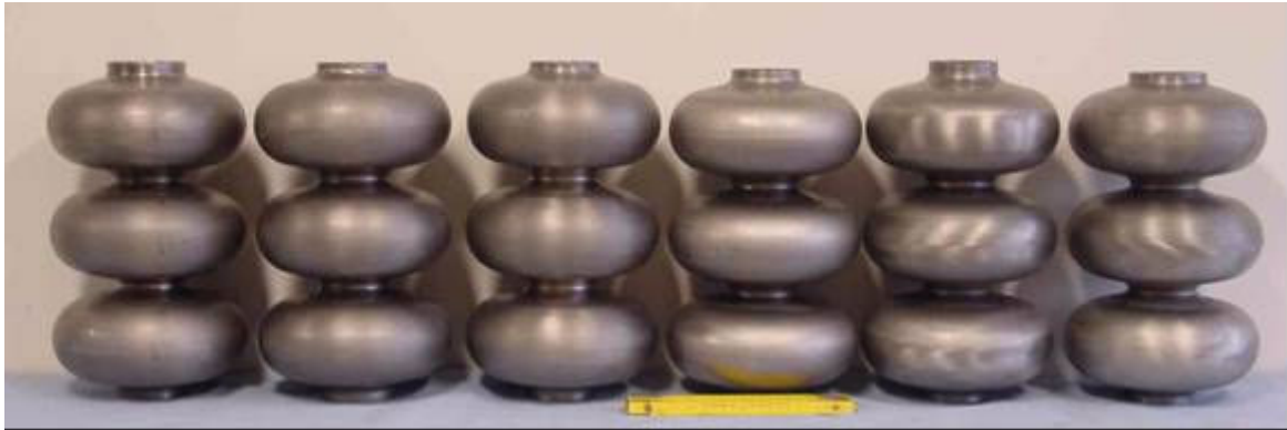
Fig. 3.2.5: Hydro-formed three cell units
