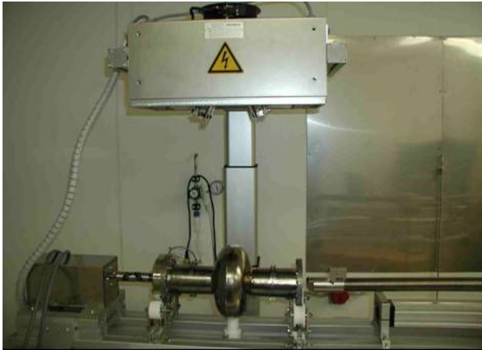
Figure 5.4.3: Dry-ice cleaning system with the new IR heater
