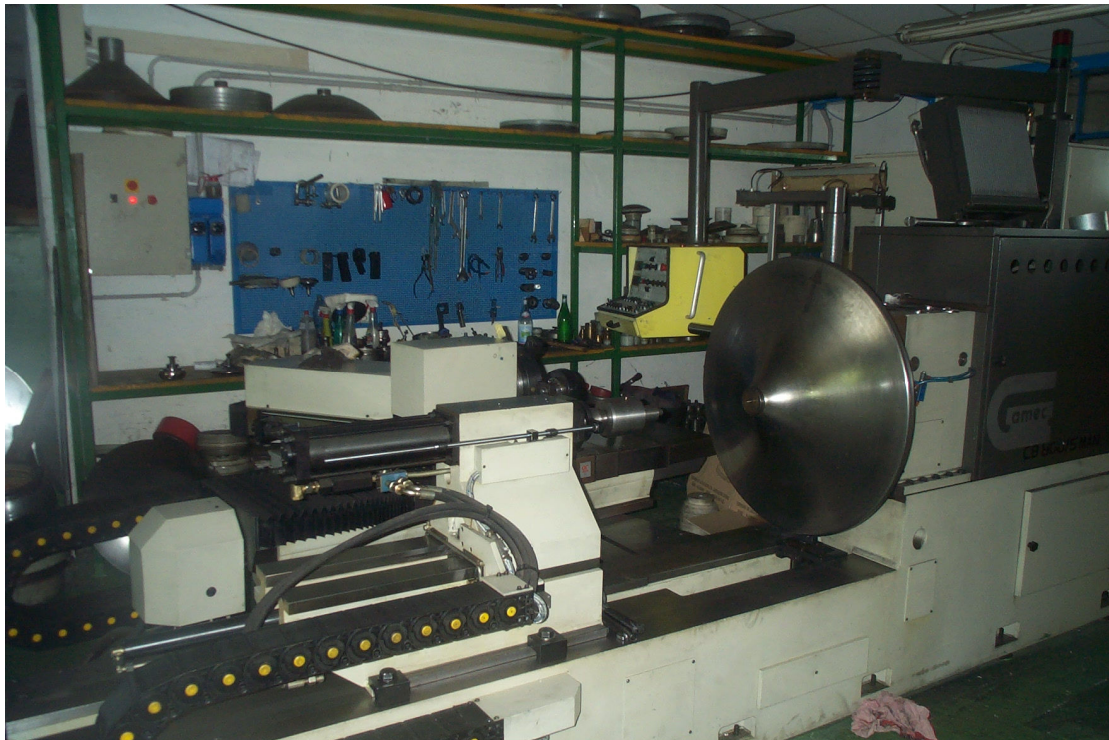
Fig. 1: The spinning lathe used for the fabrication of seamless cavity prototypes. The lathe had only one turret which hold the rollers.
