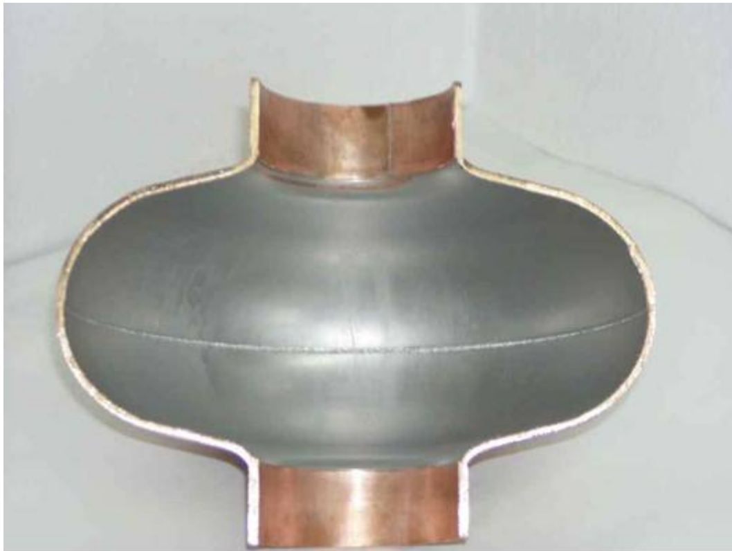
Fig.1. Inner surfaces of a single cell, which have been coated without any micro-droplet filtering
