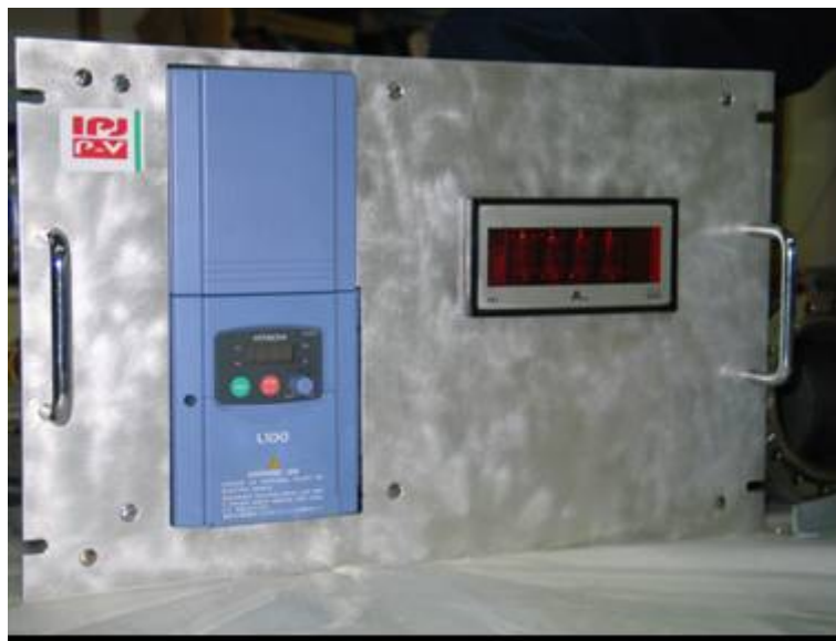
Fig.4. High-current supply unit for the cylindrical magnetic filter.
