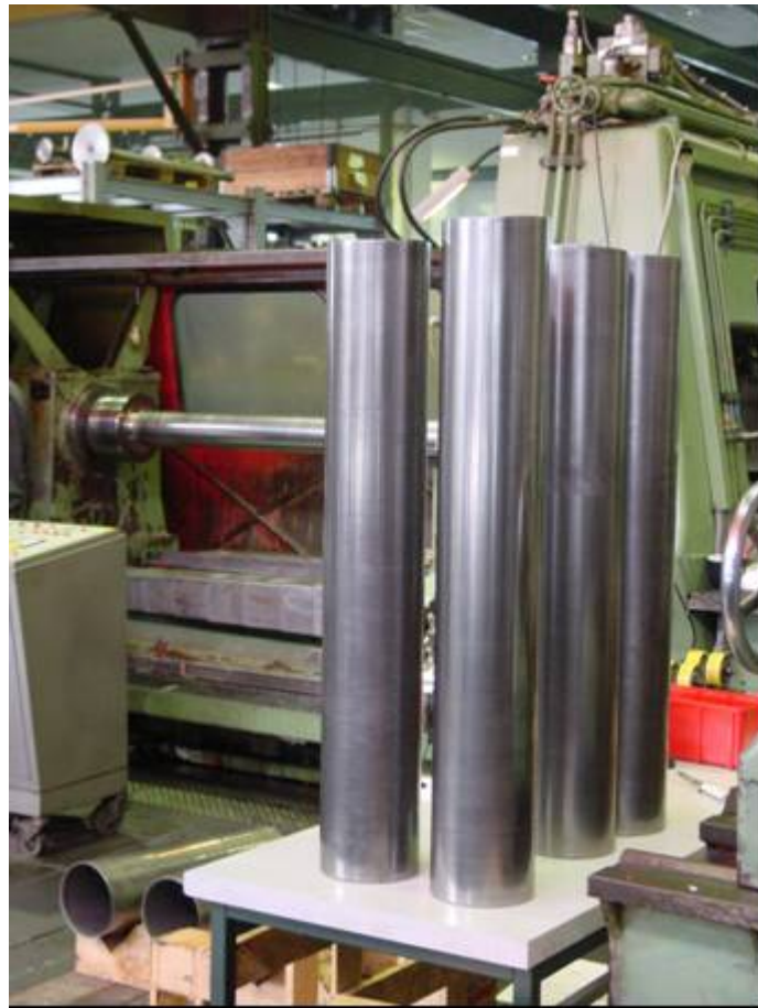
Fig. 2 Seamless niobium tubes for cavity fabrication by hydroforming
