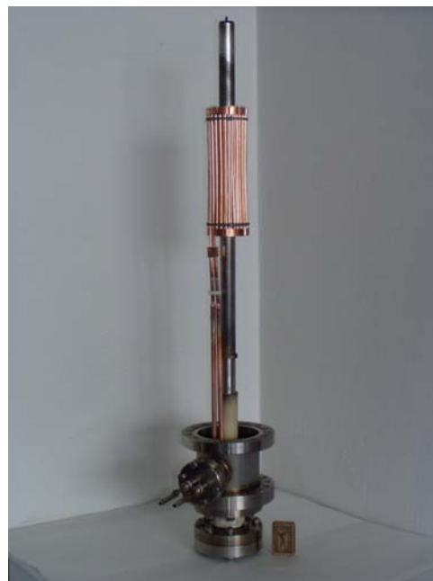
Seite 227 Fig.3. The cylindrical magnetic filter fixed upon the linear (cylindrical) cathode.
