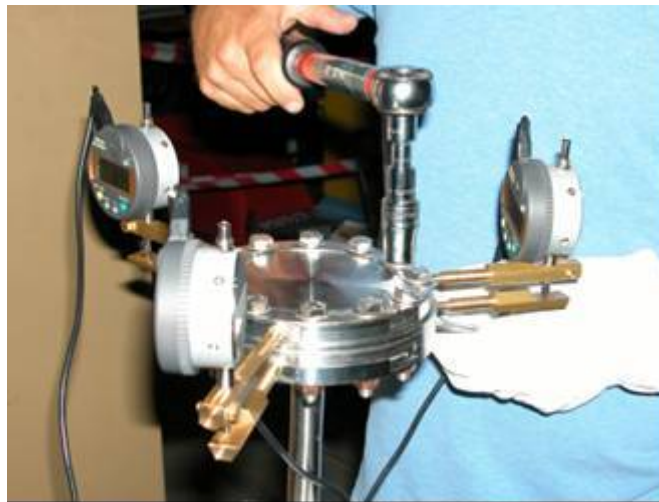
Figure 5: bolt tightening with torque meter. Displacement is measured by three gages.
