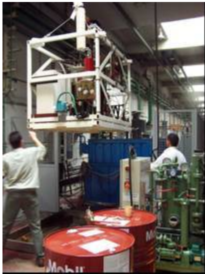
Fig.1 After cleaning, the klystron-modulator components are transferred in the oil-tank refilled with 4300 litres of new oil.
