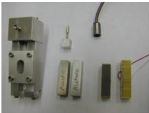
Figure 3: Device for the measurement of the thermal shrinkage
