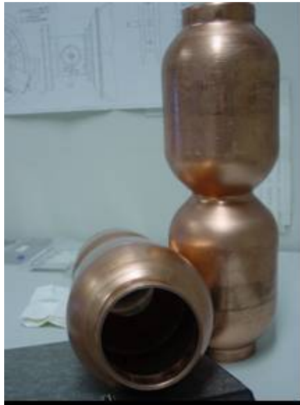
Fig. 3.4. Necking at the tube end and tube middle implemented by necking machine.
