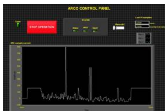
Fig.4.19. Example of arc current values recorded during operation showing automatic arc recovery.
