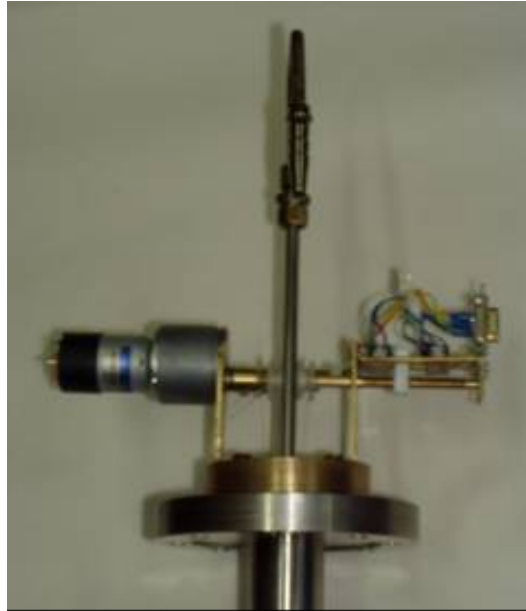
Fig. 4.6. Top part of the magnet-drive system used in the modified UHV linear arc facility.
