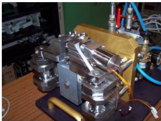
Figure 8.9. Measured stiffness on this test bench is 35 kN/mm, limited by mechanical plays in ball bearing
