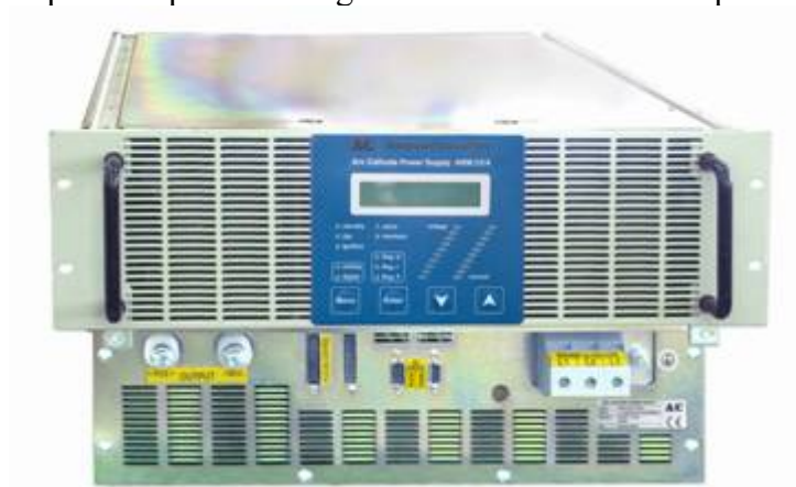
Fig 4.3. A new DC/pulse power-supply for the linear-arc facility.
