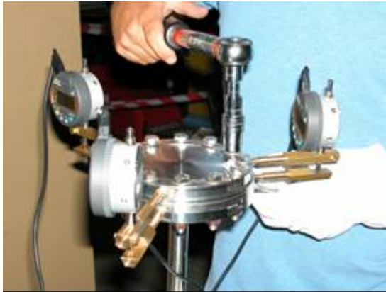
Figure 2.6: bolt tightening with torque meter and liquid nitrogen temperature leak test.
