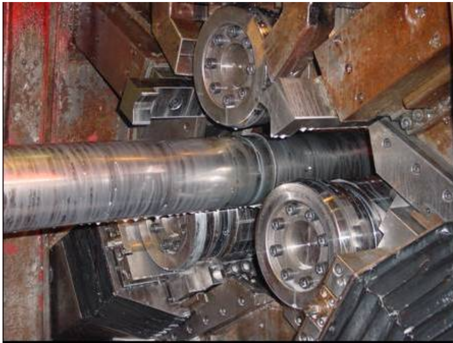
Fig. 3.7. Flow forming of the seamless niobium tubes
