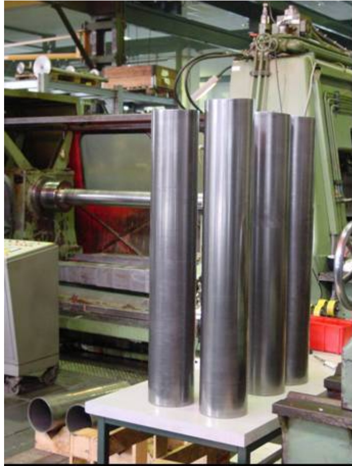
Fig. 3.6 Seamless niobium tubes for cavity fabrication by hydroforming
