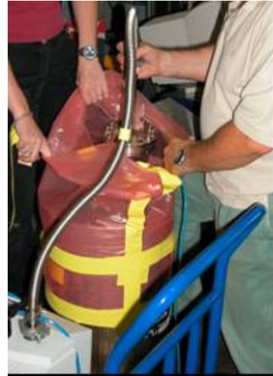
Figure 2.6: bolt tightening with torque meter and liquid nitrogen temperature leak test.
