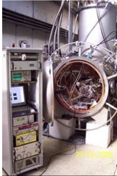
Figure 8.11. C45 TTF cavity in CRYHOLAB ready for integrated experiments. The electronics on the left allows characterization of mechanical modes of the cavity assembly: F, Q, piezo to piezo and piezo to frequency transfer functions.
