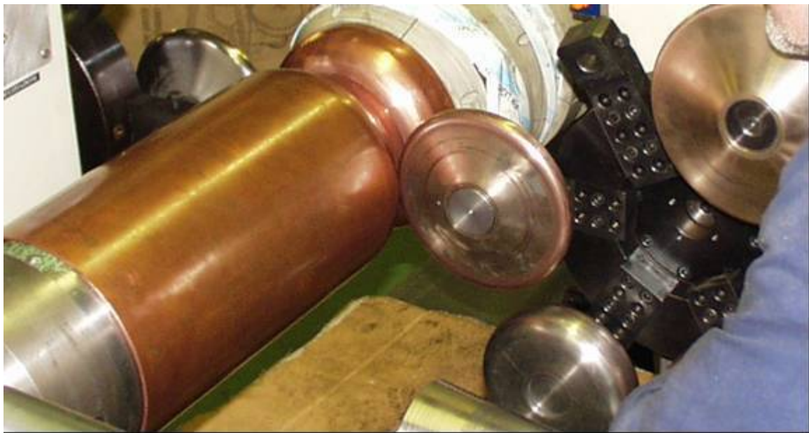
Fig. 3.1: Phase of the double turret necking process during the spinning parameter definition action.
