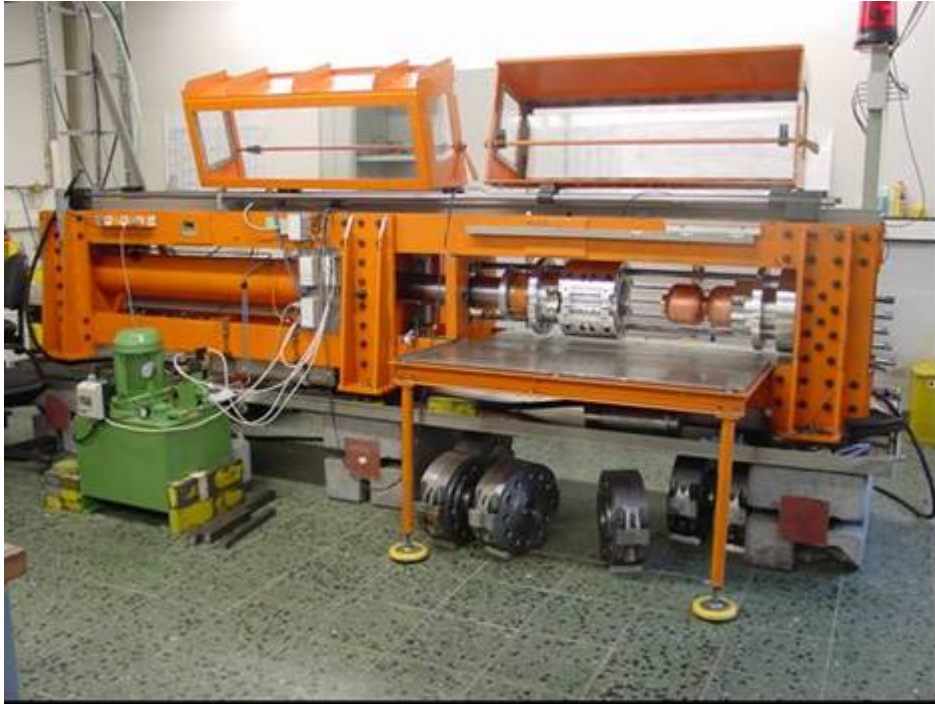
Fig. 3.5: View of the hydroforming machine
