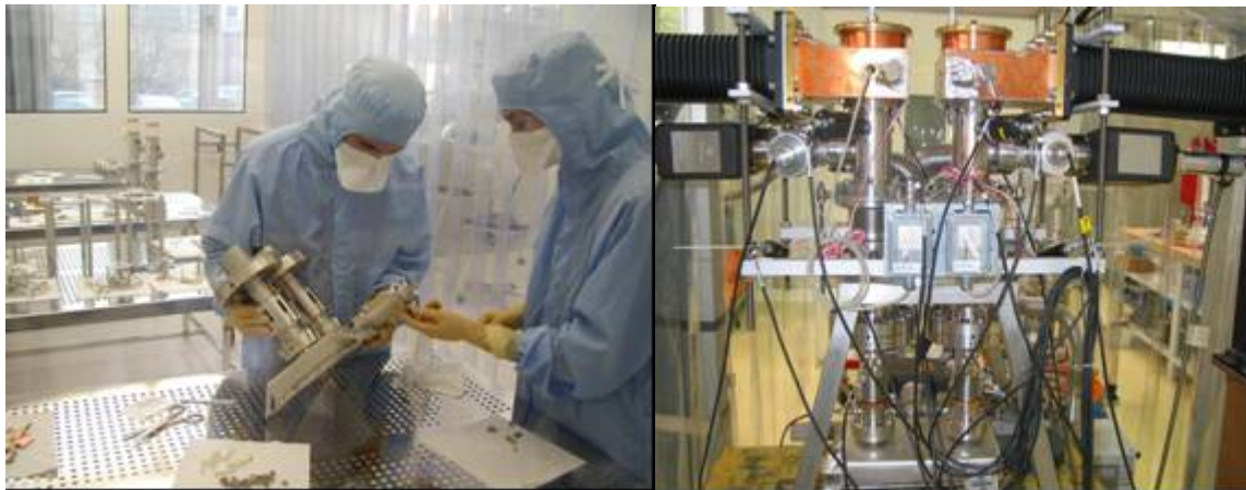
Figure 7.5. Coupler assembly in class 10 clean room. Figure 7.6. TTF-III couplers being conditioned.
