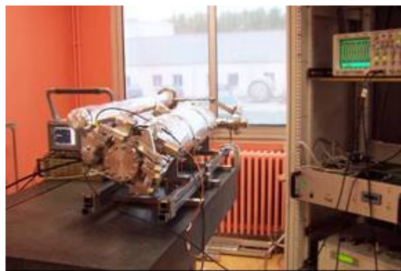
Figure 8.10. The piezo tuner is mounted on C45 TTF cavity with the electronics in the laboratory.
