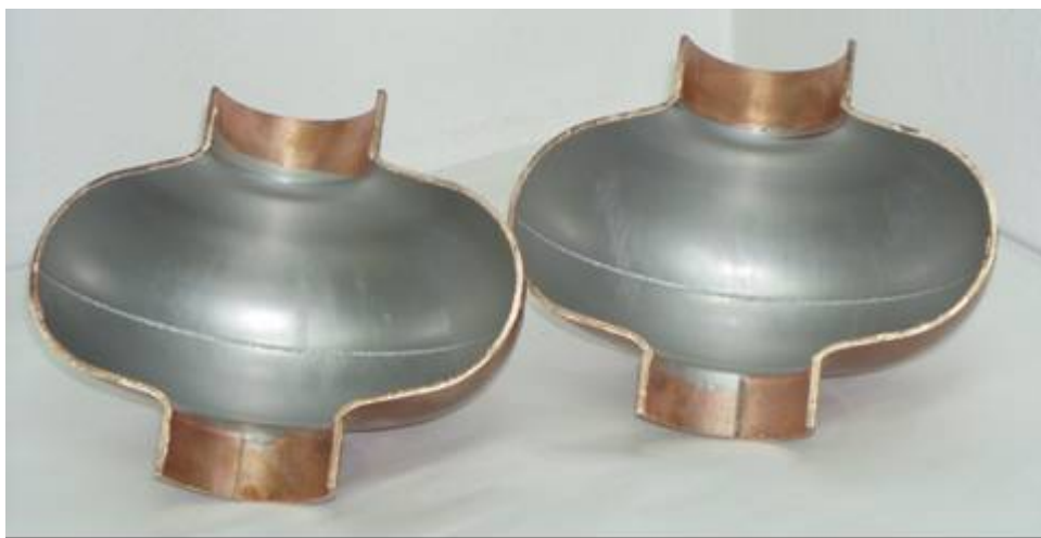
Fig. 4.7. Two parts of the coated single-cell, which was cut in order to perform an analysis of the inner surfaces.
