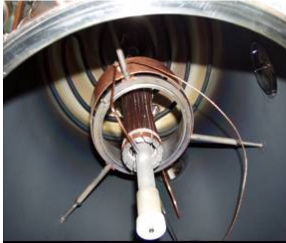
Fig. 4.12. Picture of the cylindrical magnetic filter and an additional anode after the exploitation tests.
