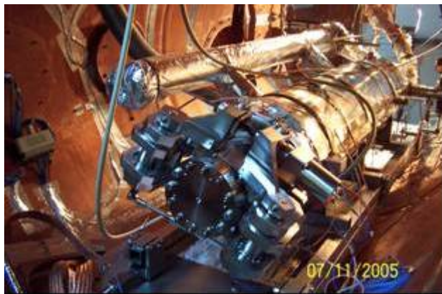
Fig. 10.3 Cold Tuning System (CTS) with Noliac Piezo Tuner mounted on 9-cell cavity for cold test in CryHoLab.
