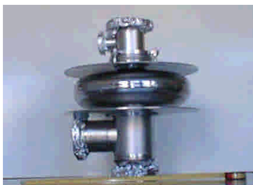
Fig. 3.12 Single cell \beta = 0.65 with the SS He-tank end caps [32]
