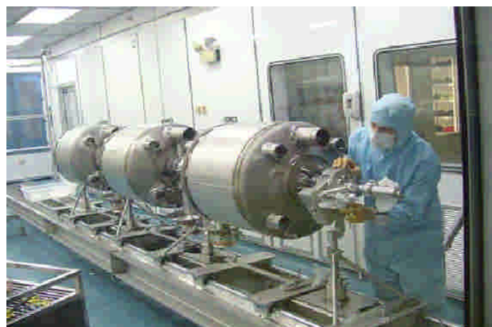
Fig. 3.9: He vessel assembling in cleaning room [31]
