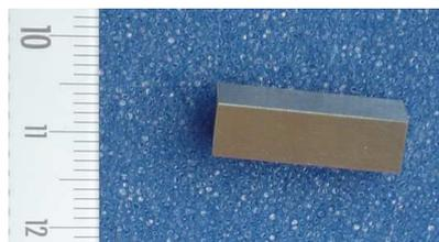
Figure 4.17 Photo of GalFeNOL rod of cross-section of 7x7 mm and length of 18 mm.
