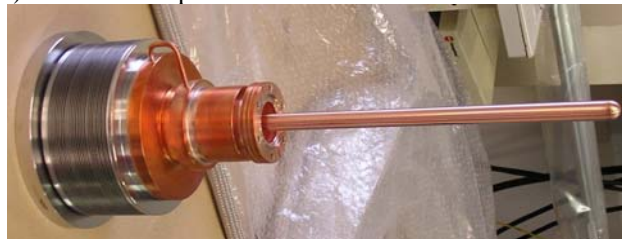
Figure 6. Proto-type of cylindrical window coupler for SPIRAL-II.
