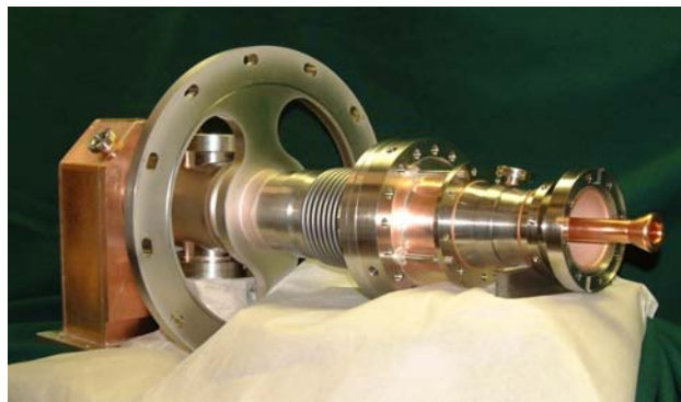
Figure 7. The AMAC coupler developed for TESLA/ILC.
