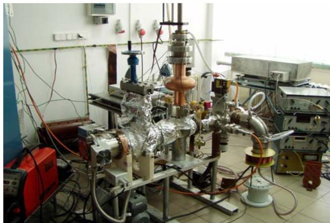
Figure 12: UHV system with a linear-arc and a test bed of the knee-shaped magnetic filter, which is operated in Swierk.
