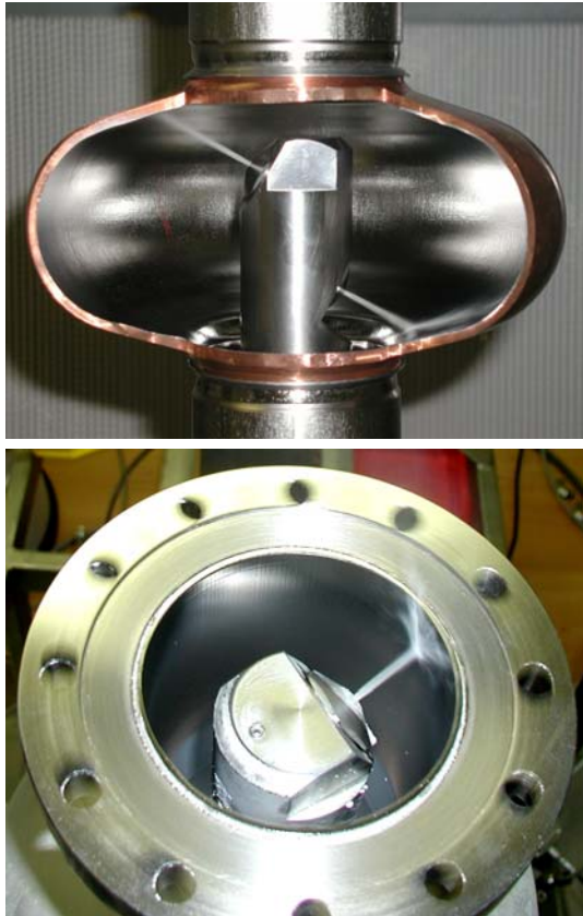
Figure 3: nozzle test in a cut NbCu cavity (top) and cleaning the beam tube of a Nb monocell (bottom)
