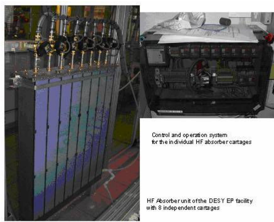
Fig. 8: Picture of the new development of gas scrubber for HF exhausting gasses
