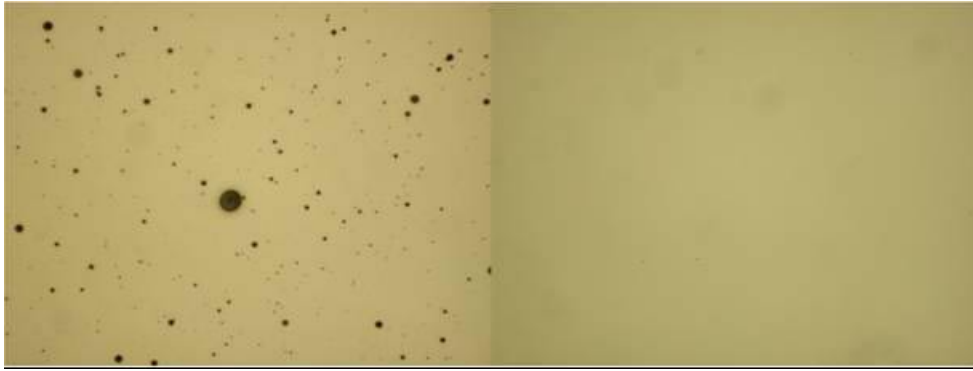
Fig.13. Microscope pictures of the identical regions ( 250 \times 190 \mu\text{m}^2 ) of the sample coated without magnetic filter (on the left) and that produced with the active filter (on the right).
