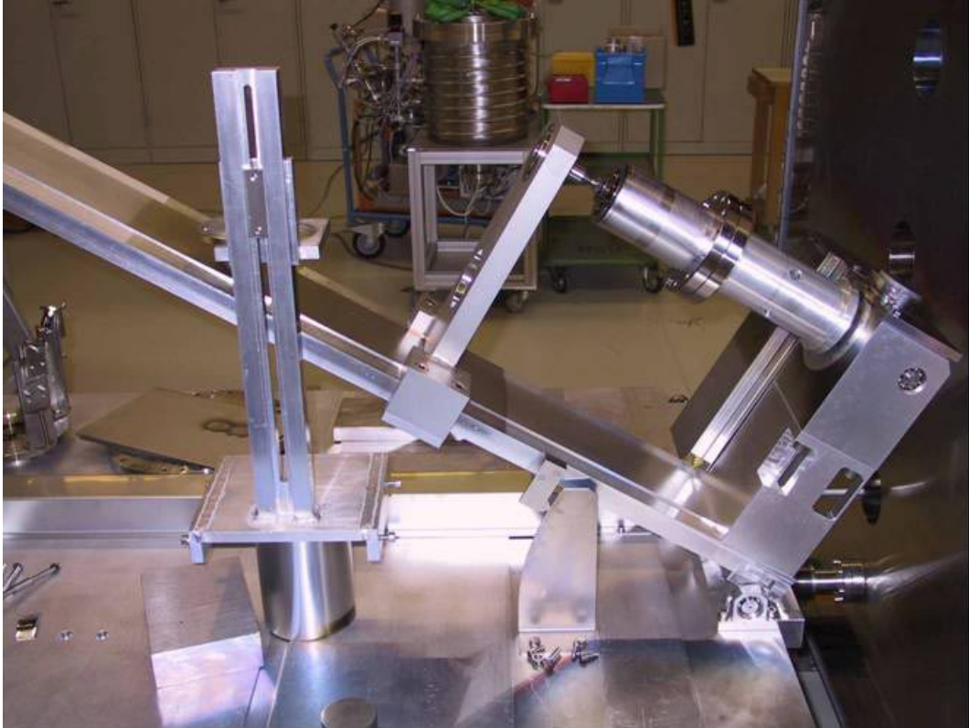
Picture 6: Welding fixture for flange-tube connections
