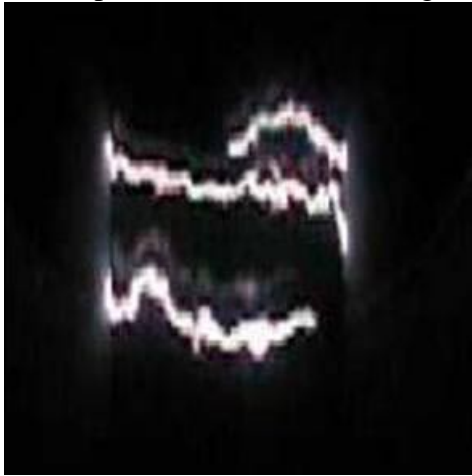
Fig.7. Picture of the linear-arc discharge upon the cylindrical cathode surface), as observed at the base pressure of 4 \times 10^{-10} mTorr, arc current of 40 A, the action lasting 1 minute.
